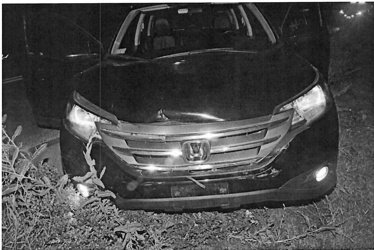
Mr Ventura's vehicle at rest near 375 Washington Avenue. Note the missing front license plate and extensive front end damage. The intersection of Washington Avenue and Fuller Street is approximately 220 feet (northbound) from the rear of Mr. Ventura's vehicle.
